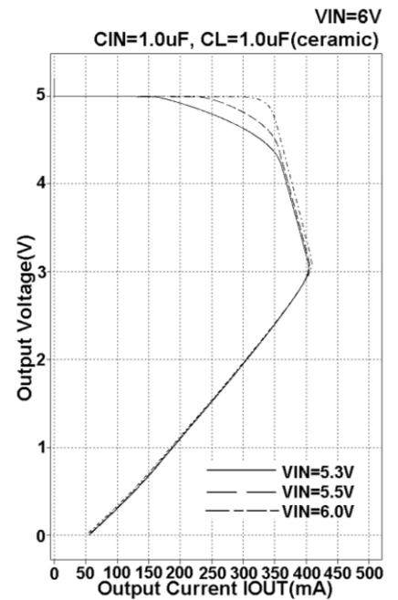
**3) Output Voltage vs. Input Voltage**
