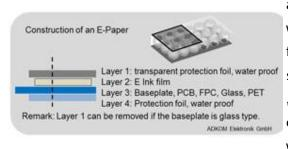
The construction of an e-paper is clearly arranged. Layer 1 represents a transparent, waterproofed protective film. The actual E INK fluid follows in layer 2. The third layer is the basic substrate, which could be made out of PCB-, FPC-, PET-material or glass. To finalize the composition, layer 4 comes in turn also with a waterproof protector. Graphic E – Paper offer high resolution and enable part addressing of the particles for multiple grayscales.
