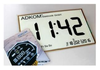
Regardless of the viewing direction this display is easy to read, even from a distance by its enormous segments. It is basically suitable for products which need to display information unchanged over a long period. In operation of the presented watch, only the segment in the second range which varies is renewed. Up to the point the clock reaches the full minute – all the segments are subject to a refresh, and are going to be renewed.
