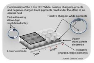
The media (beads) in turn is embedded in a fluid or light oil. By applying voltage, to represent the desired content the flakes can be drawn either to the front or back of the fluid.
